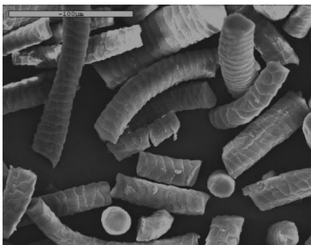
Figure 15 Structure of the wool treated under 130°C water for 3 h.
